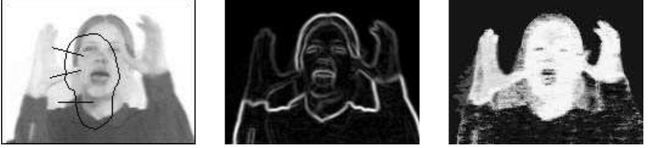
Figure 4: Left: Illustration of the search procedure. Middle and right image: Edges and skin color probability
