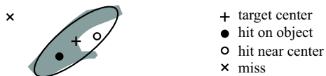
Fig. 4. Definition of tracker hit and miss with regard to target object ( grey area ). The ellipse shows a line of constant distance for quantifying tracker accuracy
